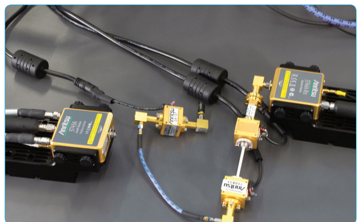
Millimeter-wave noise figure measurements with a VectorStar VNA.
